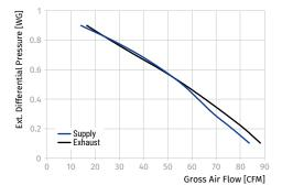
Note: fan curve performed on high speed
