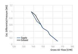
Note: fan curve performed on high speed
