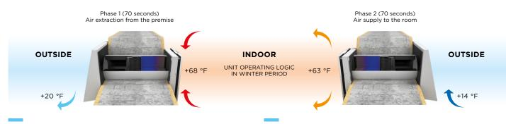
Warm stale air is extracted from the premise, flows through the ceramic regenerator and transfers its heat energy and moisture to it.
